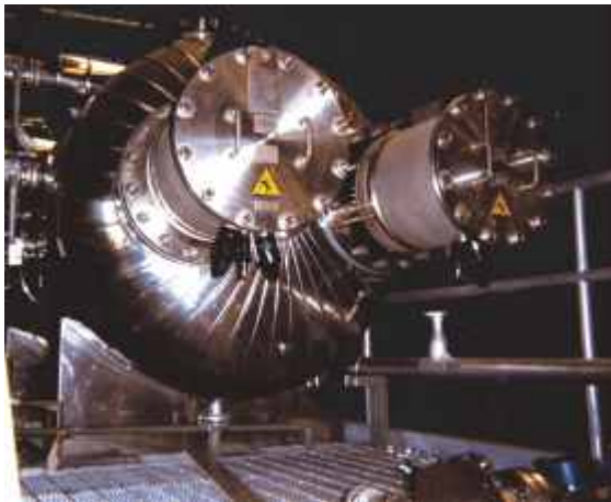
Process immersion heaters
